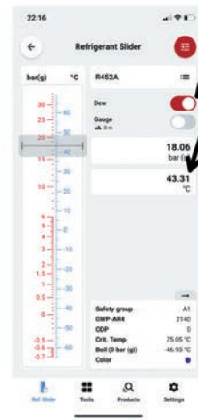
Comparator to show refrigerant properties of a zeotropic refrigerant in a condenser
