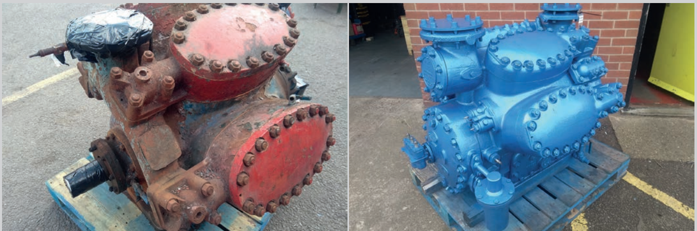
Before and after images of a V127 reciprocating compressor remanufactured by the J & E Hall team
